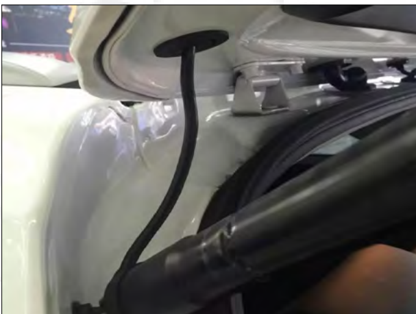
7. Pass the Holzer line through the tailgate hole (The same as the left and right steps)
