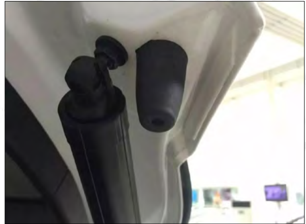
6. With the original car ball head, install the right pole. (The same as the left and right steps)
